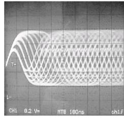
Figure 5: CD-R Recording at 32X using a thermally balanced write strategy on a phthalocyanine disc
