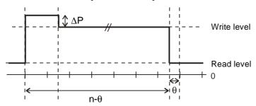
Figure 1: Write strategy suitable for CD-recording from 1X up to 4X [1]
