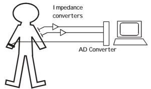
Figure 1: Set-up for contactless sensing EMG signals
