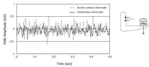
Figure 2: Recorded EMG signals with both an active- and contactless electrode
