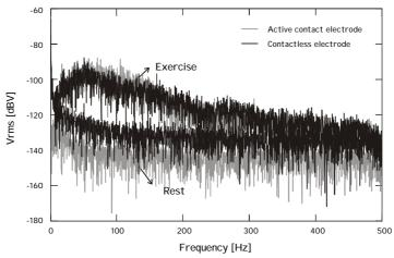
Figure 3: Spectra of the recorded EMG signals with both an active- and contactless electrode
