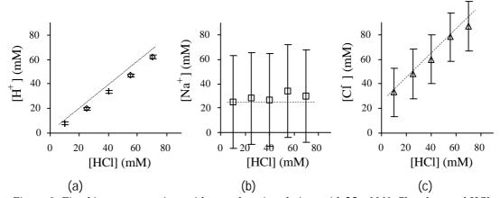
Figure 6: Fitted ion concentrations with error bars in solutions with 25 mM NaCl and several HCl concentrations. (a) H<sup>+</sup>, (b) Na<sup>+</sup> and (c) Cl
