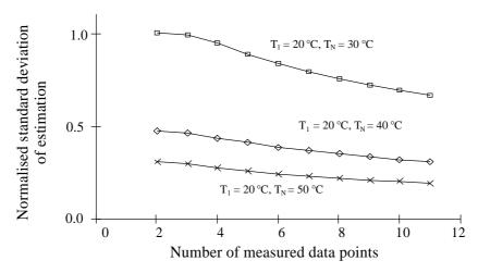
Figure 1: Effect of the temperature range and the number of measurements on the estimation accuracy
