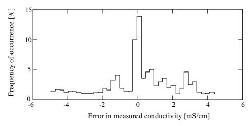
Figure 2: Error distribution in conductivity measurements
