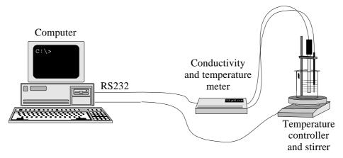
Figure 3: Measurement set-up for recording the conductivity at several temperatures
