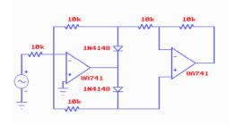
This configuration has only small diode a-linearities as shown in the transient (left) and DC (right) analysis below.
