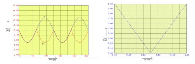
To my opinion is the noisy response in the transient analysis after a zero-crossing is due to simulation problems in Microcap. If a small a-linearity is left this is no problem in our application because this appears at the beginning of the titration curve which does not contain interesting information.
