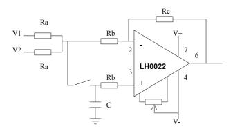
The sample and hold part in this circuitry is taken from "The National Semiconductor Cooperation Linear Applications Databook", application note AN63. The summation part is a standard method. The total output is:
