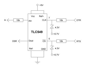
In this set-up the RS232 port is not used as it should be, but the system works on three handshake-lines. The RS232 signals may vary between -12V and +12V so zener-rectifiers are necessary to convert this signals to TTL levels. Notice that the forward potential drop across silicon based diodes is about 0.7, this would result in
