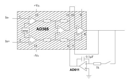
The "amp" block can be set to an amplification of 1, 10, 100 or 500 times. If the ground at the AD611 opamp is set to 2.5 volt, and the range of the output pin 8 is not larger than 2.5 volt then all possible titration curves are projected to a scale of 0..5 volt (the TLC549 input range).
