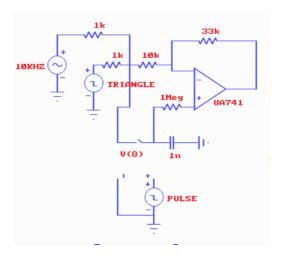
The pulse source is used to control the switch. The two input signals are a relative large triangle wave and a small sine wave (top figure). The output signal of the opamp is the sum of those two signals (bottom figure). On each sample/hold pulse, the output signal is set to zero level and starts following the sum signal again.
