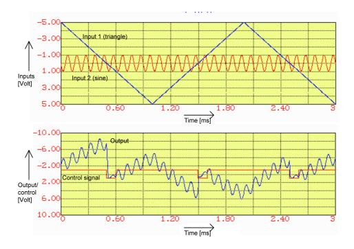
The amplification is set to  $-33k\Omega/(1k\Omega+10k\Omega) = -3$ . The voltage shift (for projecting the output range of this circuitry to the input range of the AD-converter) can be implemented by shifting the capacitor from ground.
