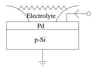
Fig. 3.7: Hydrogen gas sensor using a Pd Shottky diode
