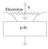
Fig. 3.6: The doped semiconductor-electrolyte device
