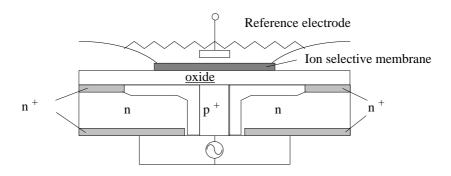
Fig. 3.10: The ICD using a lateral bipolar transistor  $\,$
