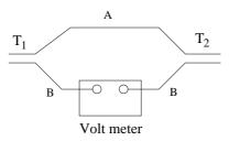
Fig. 4.3: Measurement of a Seebeck thermoelectric emf
