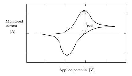
Fig. 3.3: Schematic drawing a cyclic voltammogram
