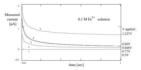
Fig. 3.1: Calculated example of chronoamperometric experiment
