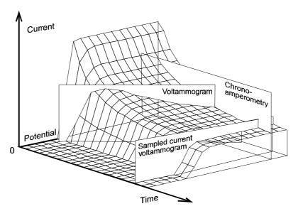
Fig. 3.4: Some controlled potential techniques in one i(v,t)-graph
