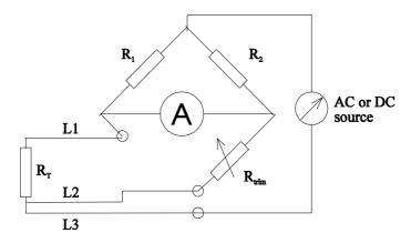
Fig. 4.1: A three-wire Pt100 element in a bridge circuitry
