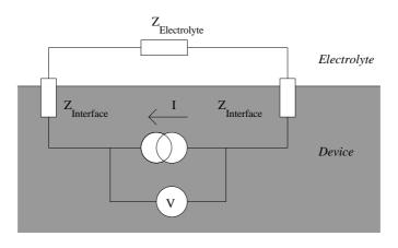
Fig. 4.7: Conductivity measurement in two point set-up
