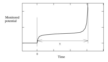
Fig. 3.5: Chrono potentiometry and the transition time t
