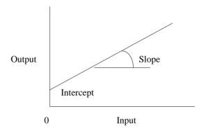
Fig. 2.1: Simplistic representation of a transducing mechanism
