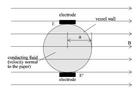
Fig. 4.5: Principle of electromagnetic flow meter
