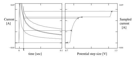
Fig. 3.2: Schematic drawing of sampled current voltammogram
