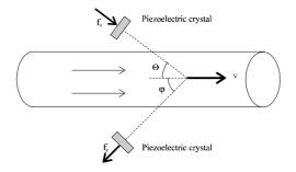
Fig. 4.6: Set-up of a Doppler shift measurement
