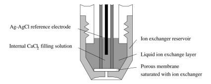
Fig. 4.9: Liquid membrane calcium electrode
