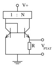
Fig. 4.4: A practical PTAT temperature sensor set-up
