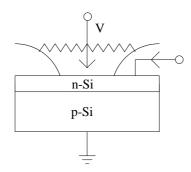
Fig. 3.8: pn-Junction used for the transistor technique
