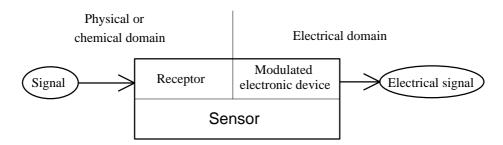
Fig. 1.2: Basic structure of a sensor
