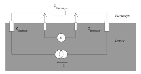
Fig. 4.8: Conductivity measurement in four points set-up
