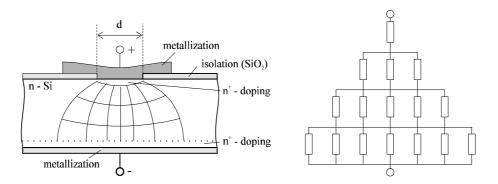
Fig. 4.2: Spreading resistance measurement device and equivalent circuit [29]
