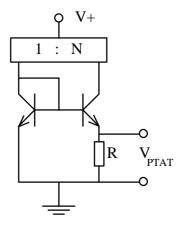
Figure 5.1: A PTAT temperature sensor
