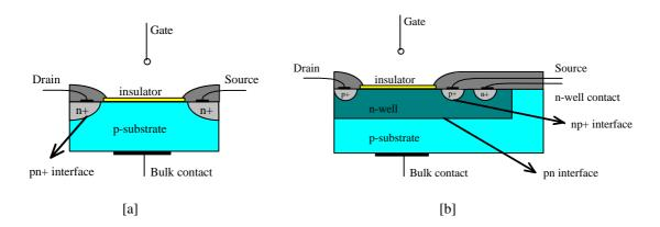
Figure 9.1: Diode interfaces in ISFETs
