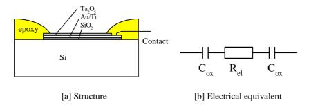
Figure 7.1: The Ta<sub>2</sub>O<sub>5</sub> electrode
