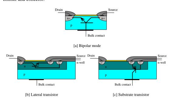
Figure 9.2: Bipolar modes in ISFETs
